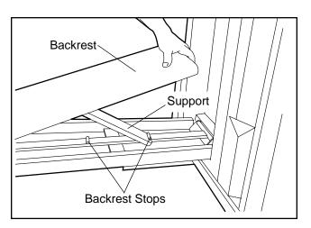
of the backrest stops as shown. Make sure that the support is resting against one of the backrest stops.
